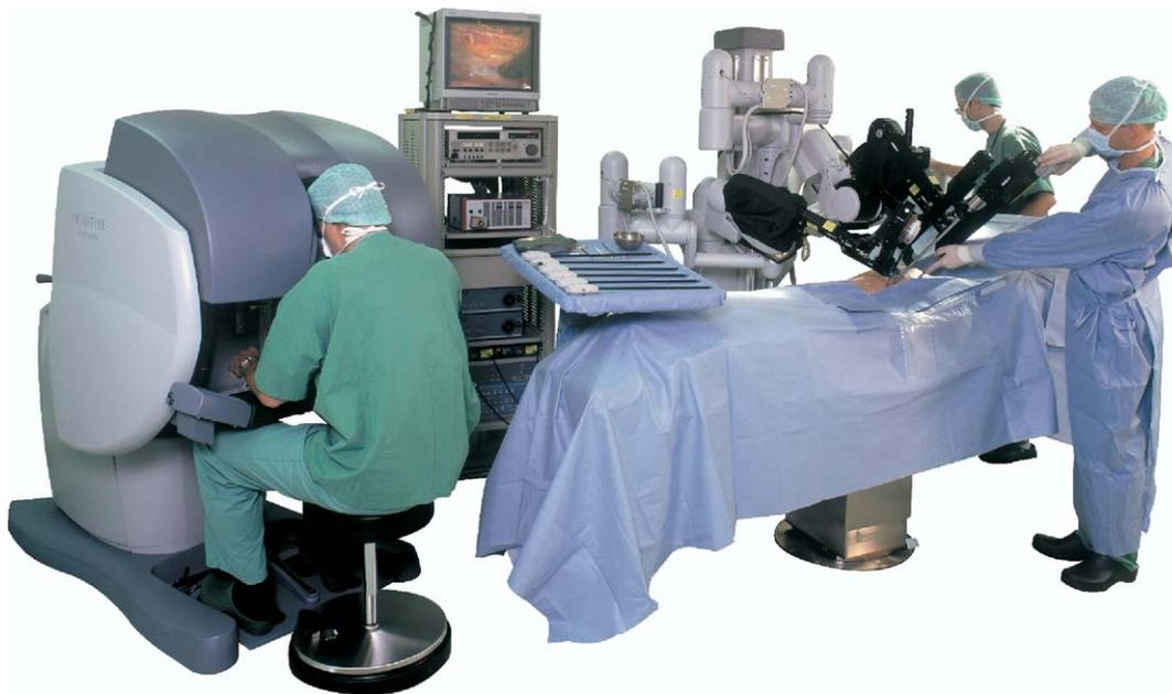
**Figure 1** The surgeon controls the da Vinci robot from a computer console positioned remotely away from the patient. The robotic tower, wheeled into the side of the operating table, supports robotic arms. The central arm serves to maintain the video telescope (12 mm diameter), which contains two separate 4-mm scopes that provide the surgeon a three-dimensional view. The remaining arms hold surgical instruments (8 mm diameter). © 2006 Intuitive Surgical, Inc.
